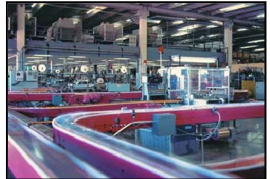
Additional equipment in the tea-packing area includes box machines, tea-bag machines, box-closing machines, overwrap machines, and case packers, as well as robots that take the cases and put them on pallets. Employees take great care to ensure that they meet the company's goal of producing only the highest quality teas.
