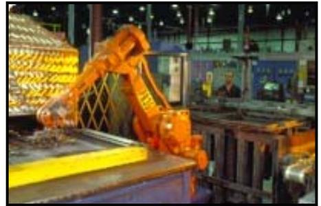
Robinson explains that "sintering" is the name of the part of the process used to build vehicle components. "Imagine a bucket filled with wet sand. When you turn the bucket over, the sand stays in place. That's similar to how we build our vehicle parts. We take powdered metals and press them together with several hundred tons of force. Then presto — the part is ejected."
